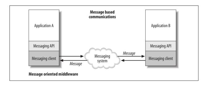
Figure 9: Communication in a MOM. Picture taken from [6]
